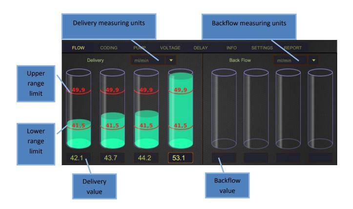
This section used to measure flow and backflow of injectors.
