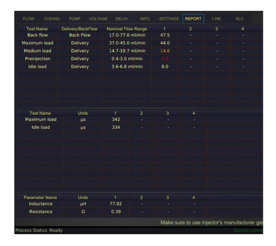
During the injectors test in AUTO or TESTPLAN mode, or during the pump test in TESTPLAN mode, a result report is generated. The first are the results of the flow tests; the data of the injection delay is in the middle; resistance, capacitance and inductance measurements are located at the bottom of the report.
