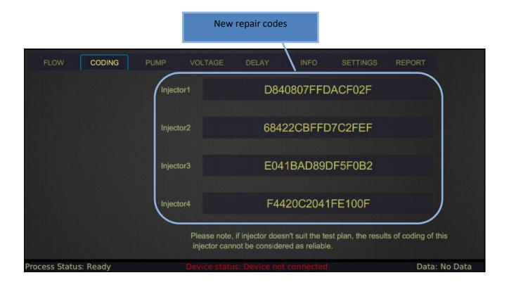
To start the assignment of codes to injectors, you need to choose CODING mode in the main section, select manufacturer, injector number and start the test with the START / STOP button in the main section. Upon completion of the coding process, new repair codes are displayed in this section.
