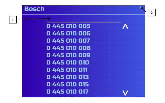
(1) Filter is a line for inputting a part of a serial number to simplify search in the database. Data base records, which do not contain the inserted part of the number, will be automatically removed from the screen.
