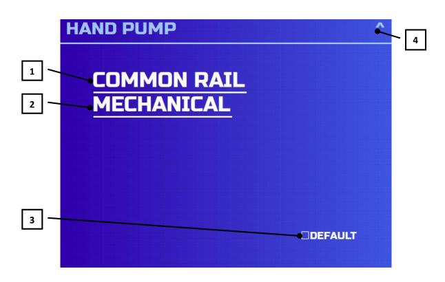
(1) COMMON RAIL – testing of Common Rail injectors on the hand pump (express test).
