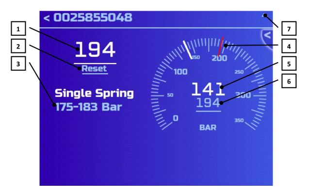
(1) **Opening injector pressure** – fixed pressure of the injector opening.
