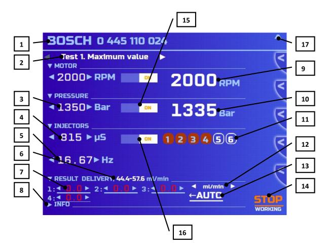
(1) Information line is a line where manufacturer and serial number of tested injectors are shown.
