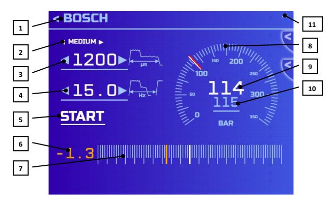
(1) Type of the tested injector.
