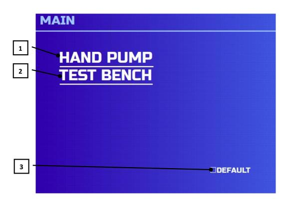
(1) HAND PUMP is a mode for testing mechanical and common rail injectors with the hand pump.
